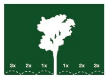
Kauri Tree Measure the outermost canopy dripline and multiply three times in a radius around the trunk.
